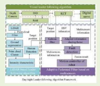
Researchers at Shandong University in China have recently developed a new framework that could provide four-legged robots with leader-following abilities in both nighttime and daytime conditions. This framework, introduced in MDPI's Biomimetics journal, is based on visual and LiDAR detection technology.
